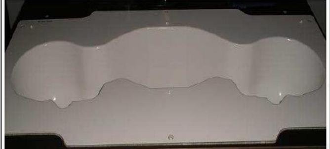
The bottom plate contains three pair of bolts for locking the device holder. The device holder positions are adjusted to the standard measurement positions in the three sections. A white cover is provided to tap the phantom during off-periods to prevent water evaporation and changes in the liquid parameters. On the phantom top, three reference markers are provided to identify the phantom position with respect to the robot.
