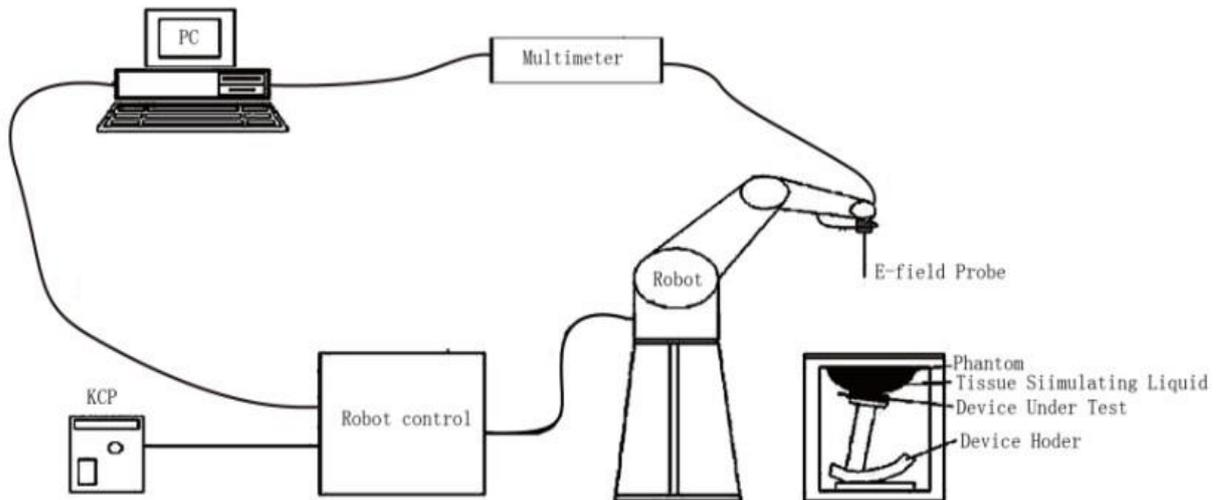
The COMOSAR system for performing compliance tests consists of the following items:
