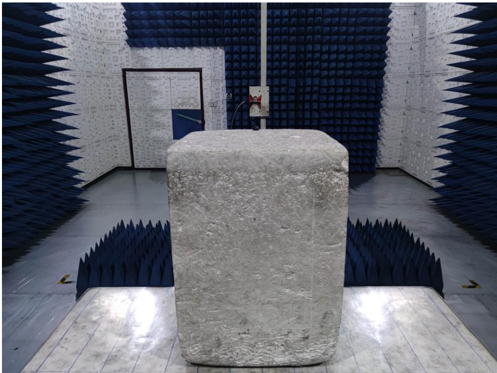
RADIATED EMISSION TEST SETUP ABOVE 1GHz
