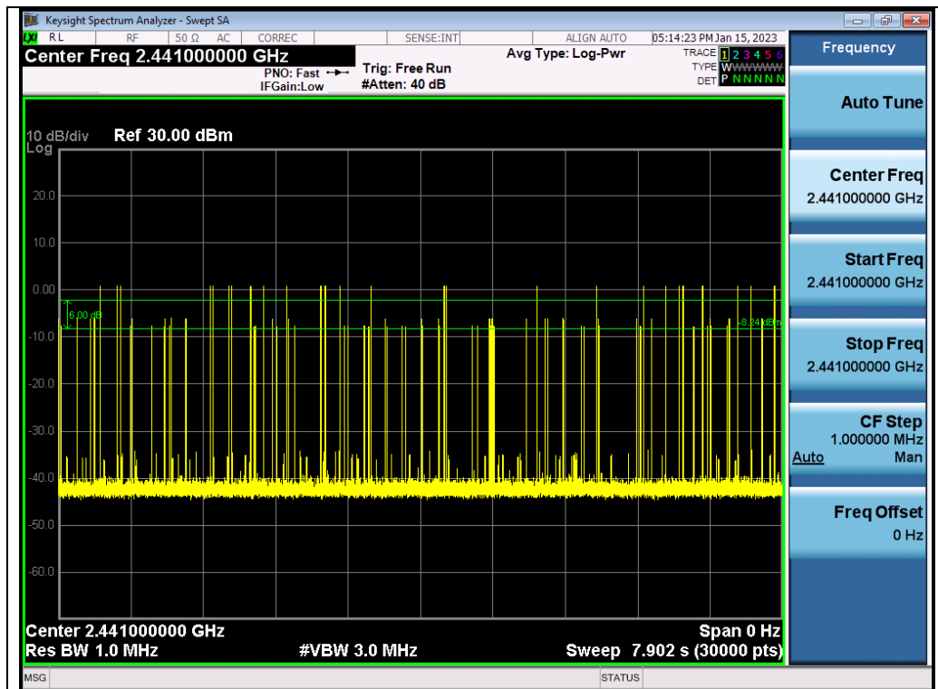
Test_Graph_BR_HOP_ANT1_NA_1Mbps_2441_Number of Burst
