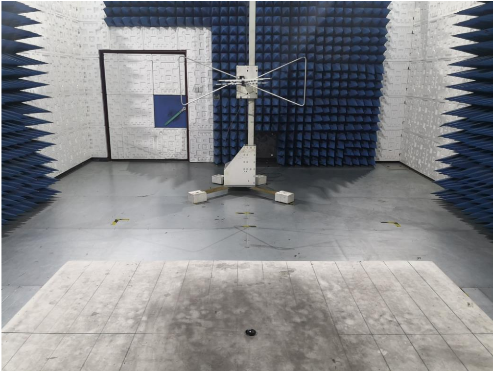
RADIATED EMISSION TEST SETUP ABOVE 1GHZ
