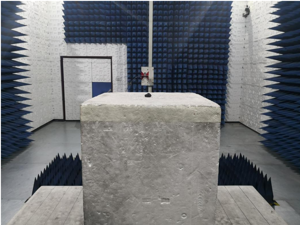
RADIATED EMISSION TEST SETUP ABOVE 1GHZ
