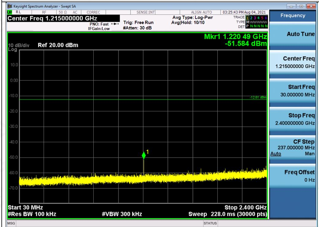
Test\_Graph\_EDR\_ANT1\_2441\_2Mbps\_Lower Band Emissions
