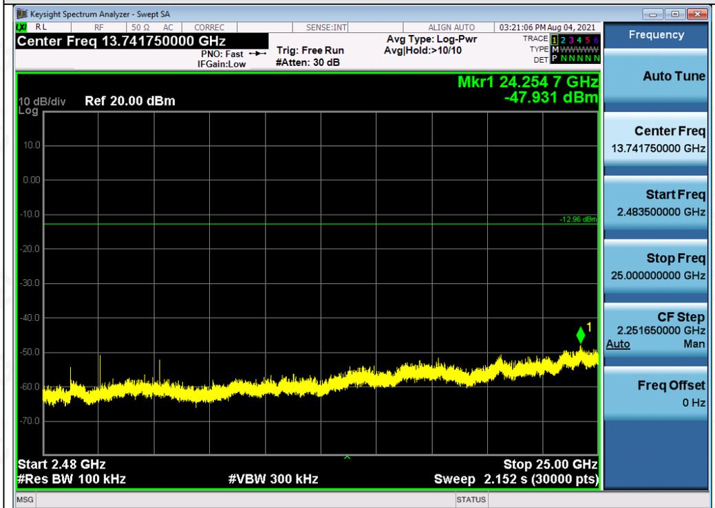
Test\_Graph\_EDR\_ANT1\_2402\_2Mbps\_Higher Band Emissions
