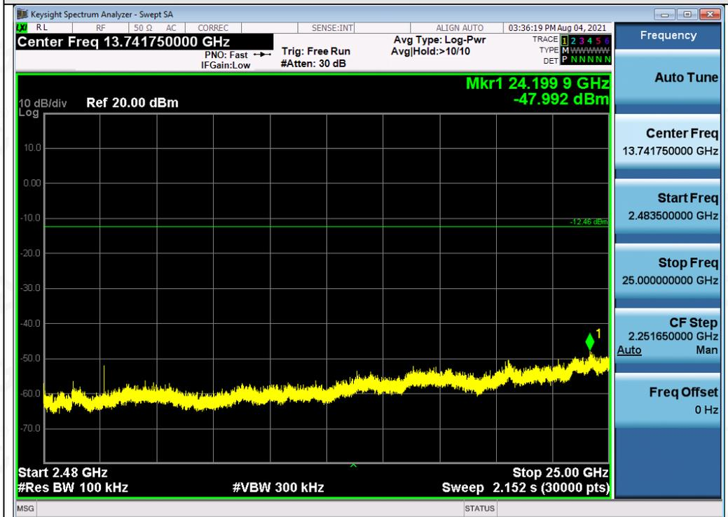
Test\_Graph\_EDR\_ANT1\_2441\_3Mbps\_Higher Band Emissions
