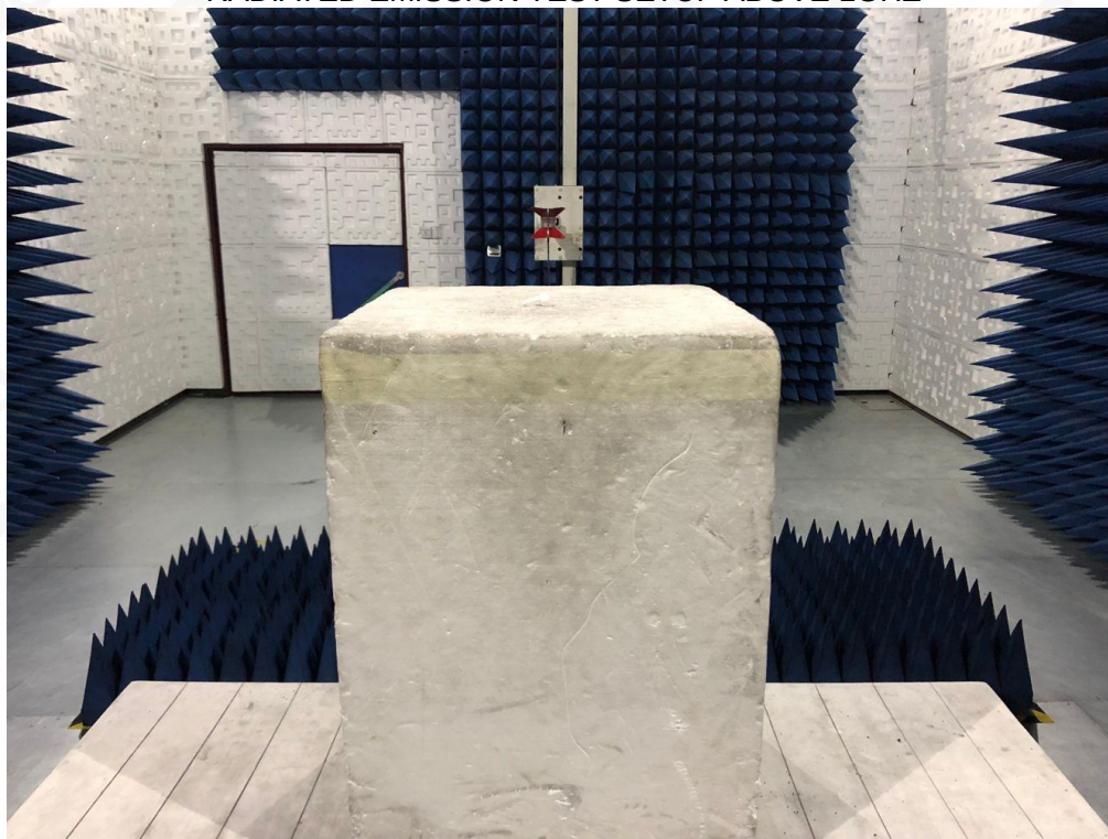
RADIATED EMISSION TEST SETUP ABOVE 1GHZ
