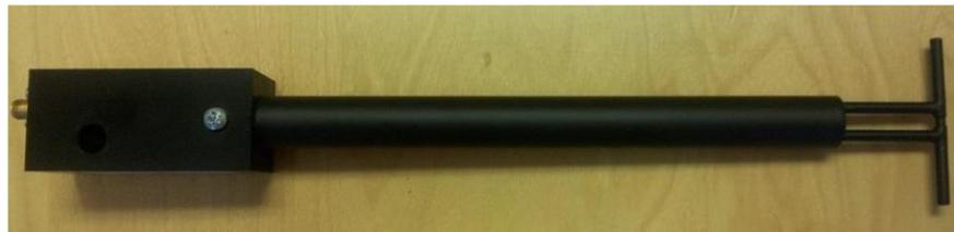
**Figure 1 – MVG COMOSAR Validation Dipole**
