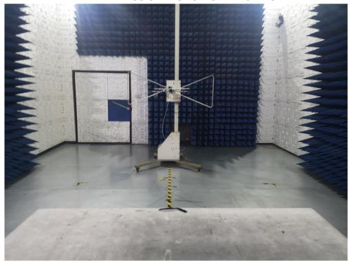
RADIATED EMISSION TEST SETUP ABOVE 1GHz
