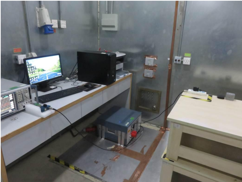
FCC RADIATED EMISSION TEST SETUP
