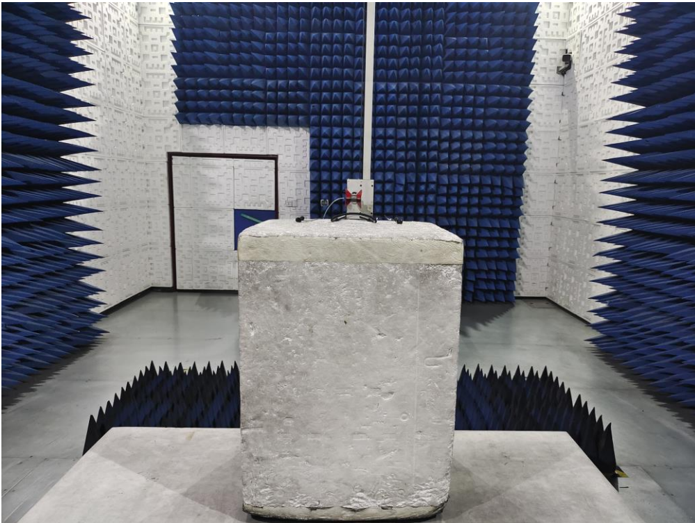
RADIATED EMISSION TEST SETUP ABOVE 1GHz
