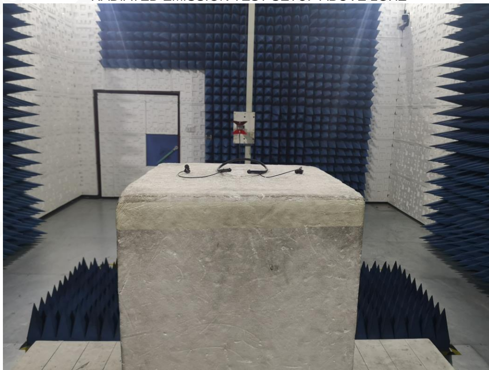
RADIATED EMISSION TEST SETUP ABOVE 1GHZ
