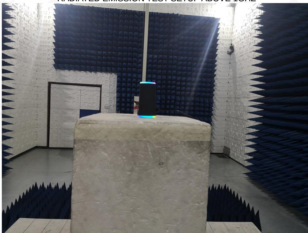
RADIATED EMISSION TEST SETUP ABOVE 1GHZ
