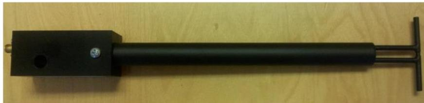
**Figure 1 – MVG COMOSAR Validation Dipole**
