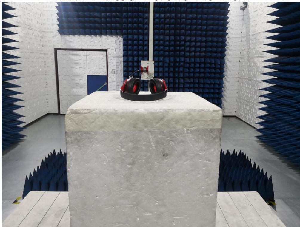
RADIATED EMISSION TEST SETUP ABOVE 1GHZ
