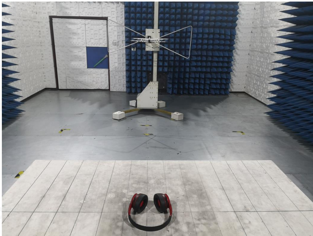
RADIATED EMISSION TEST SETUP ABOVE 1GHZ
