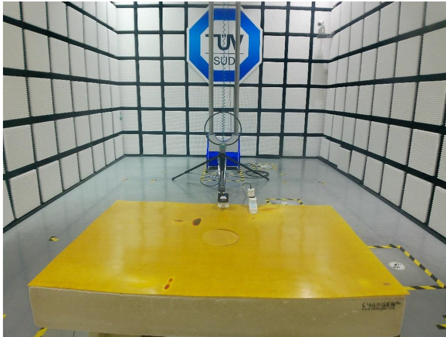
Radiated Emission Test below 30MHz
