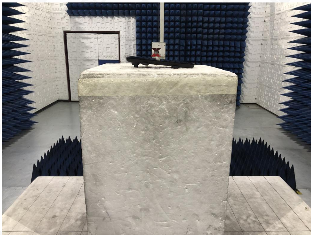
FCC RADIATED EMISSION TEST SETUP ABOVE 1GHZ
