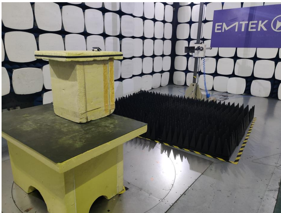
Spurious Emission Test Setup (Above 1GHz)
