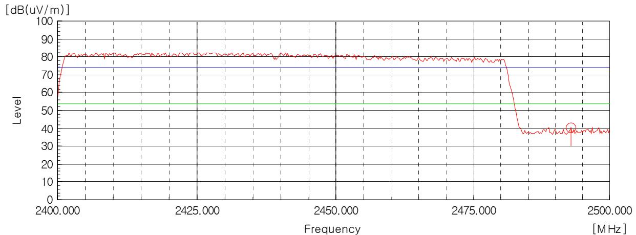
AV Detector: RBW: 1 MHz, VBW: 10 Hz (2 483.5 MHz - 2 500.0 MHz), Worst case (High, Vertical)
