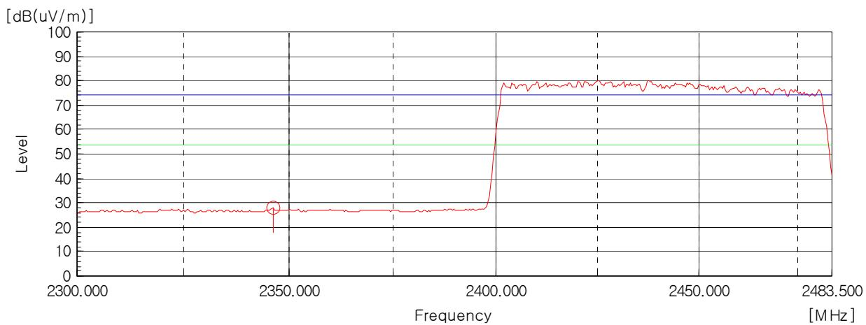
Peak Detector: RBW: 1 MHz, VBW: 1 MHz (2 483.5 MHz - 2 500.0 MHz), Worst case (High, Vertical)
