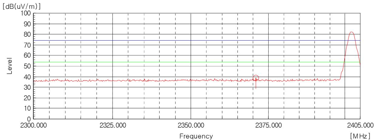
AV Detector: RBW: 1 MHz, VBW: 10 Hz (2 310 MHz - 2 390 MHz), Worst case (Low, Vertical)
