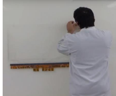
Fig.10 With the help of the “Quality approved” sticker peel the Touch Sensor protection layer
