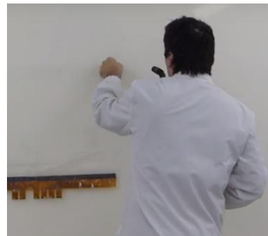
Fig.12 Start peeling off the protection layer by pulling the sticky tape together with the protection layer
