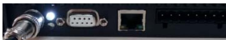
Startup normal completion after “Di” with **Power and Status LED** light, self-test completed successfully, reader is ready.
