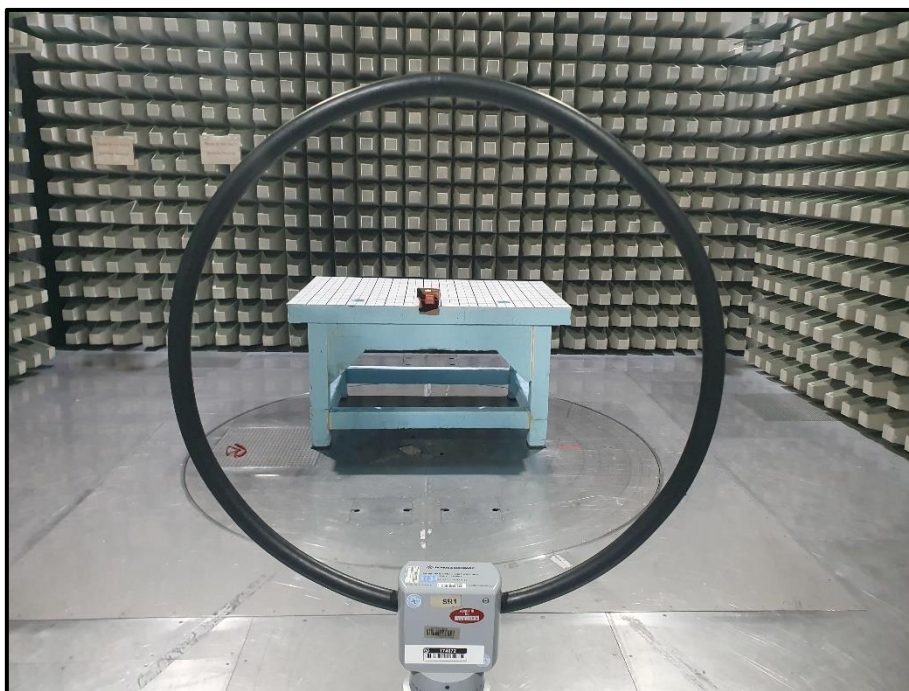
Photo 1: Radiated Test Setup-9 kHz to 30 MHz
