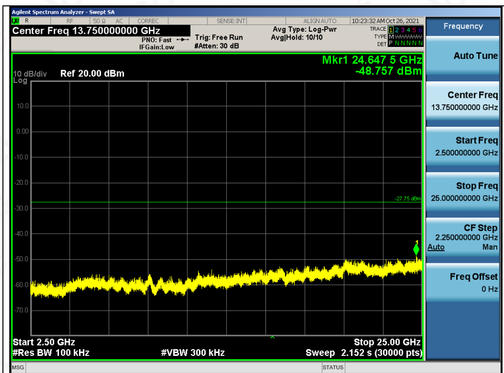
Test_Graph_BR_ANT1_2480_1Mbps_Higher Band Emissions
