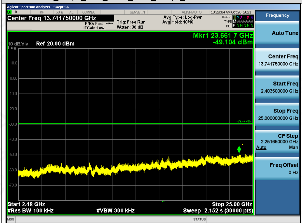
Test_Graph_EDR_ANT1_2402_2Mbps_Higher Band Emissions
