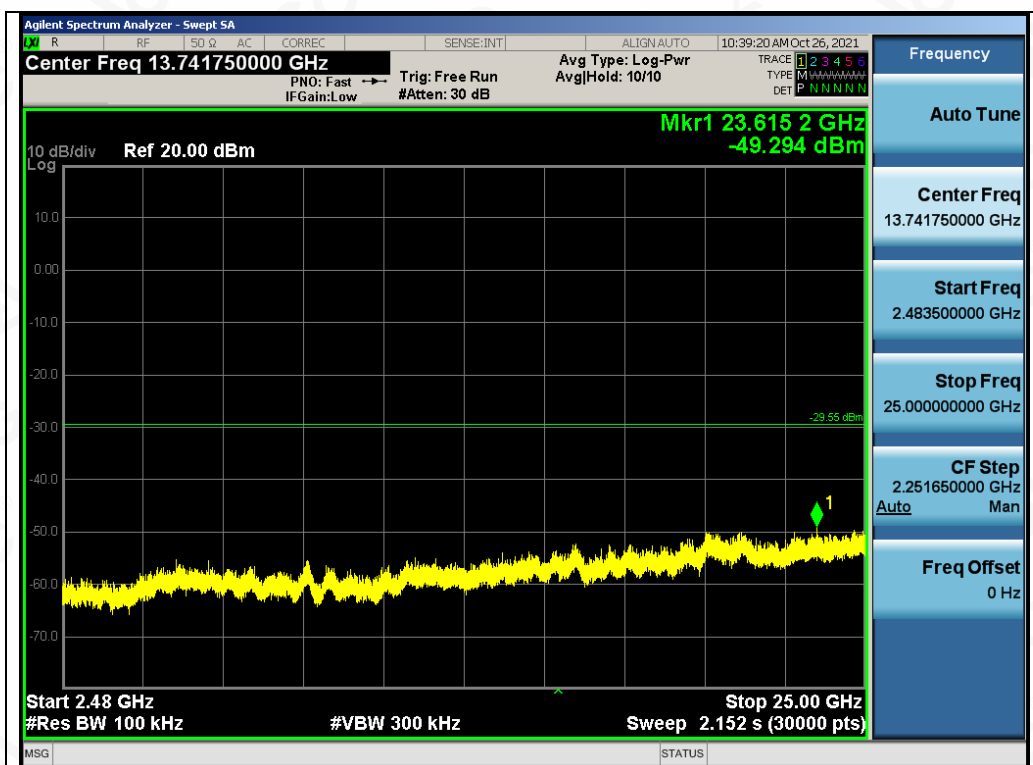
Test_Graph_EDR_ANT1_2402_3Mbps_Higher Band Emissions
