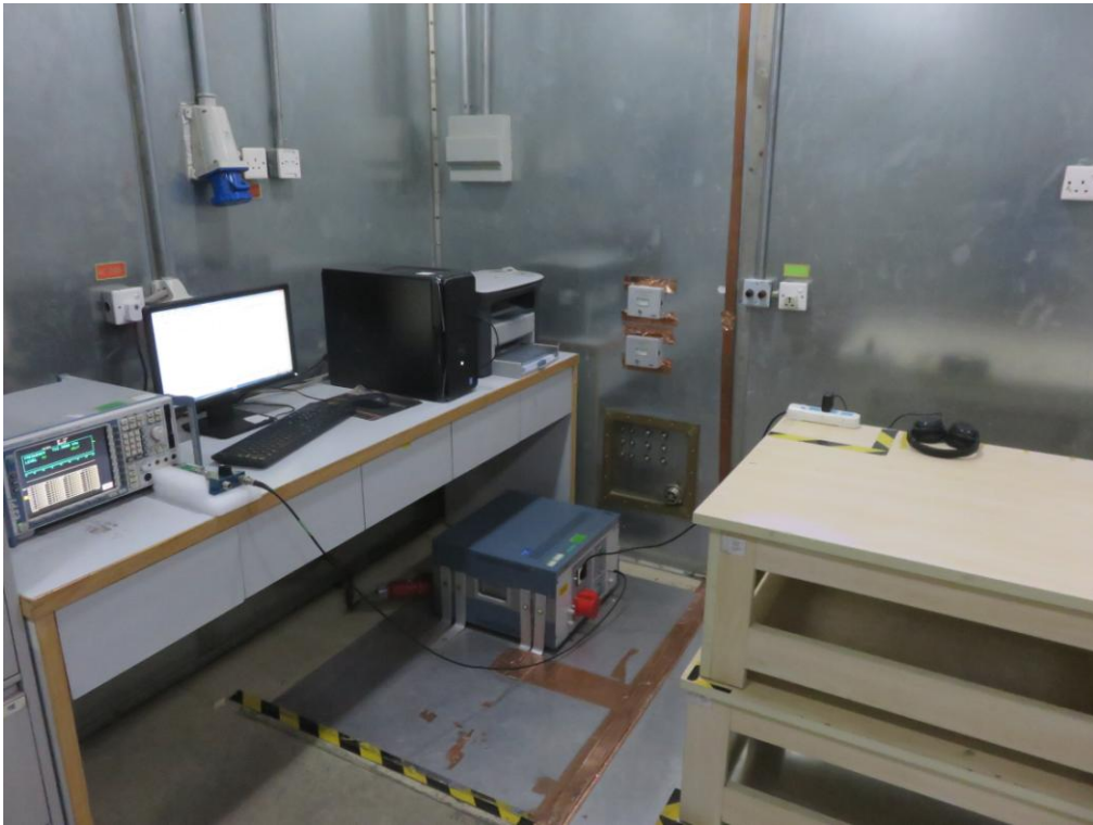
FCC RADIATED EMISSION TEST SETUP
