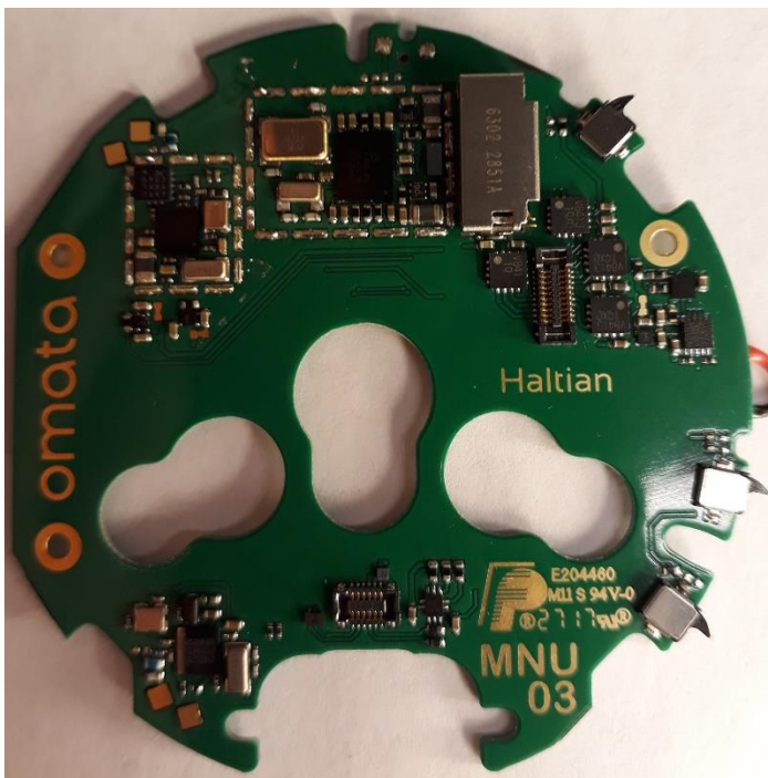
PCB without shields
