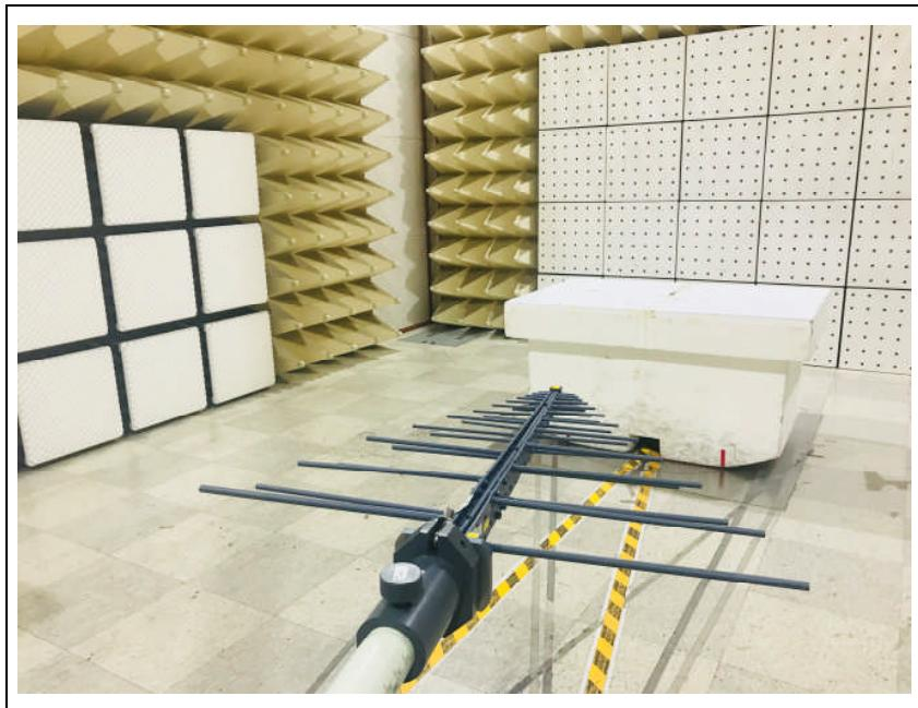
**3. Photo of Radiated Spurious Emission Test (Above 1 GHz)**
