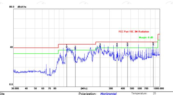
Site Limit: FCC Part 15C 3M Radiation Polarization: Horizontal
