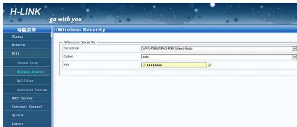
Figure 3.1.6 Setting the wireless network safe password
