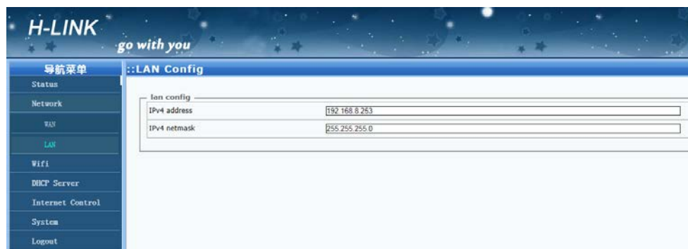
Figure 3.1.3 Setting the IP address of the LAN port
