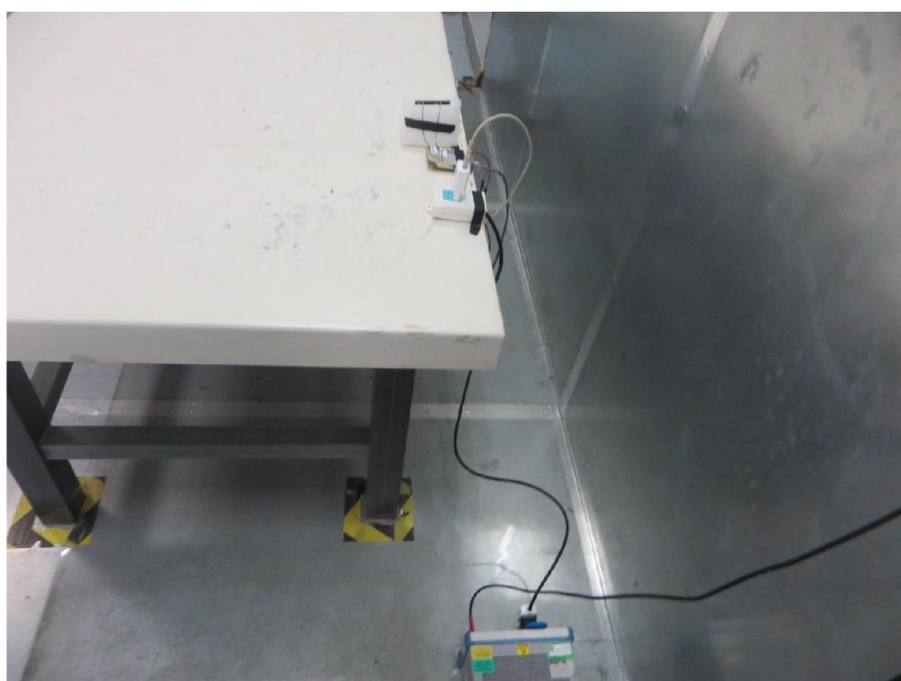
**Note: For Radiated Emission, the edge of test table align with the center of turn table.**
