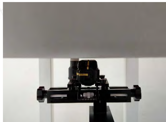
Fig.4 EUT Top side to flat phantom
