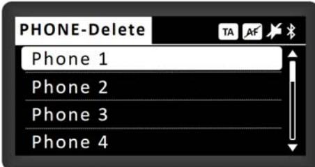
**PHONE-DELETE** screen is deleting an already paired (before paired) phone from radio paired list. Thus, radio will not try to connect to deleted phone.
