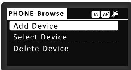
**PHONE BROWSE** screen is default screen when there is no connected device to the radio. On this screen user can add a new device, select or delete one of the devices already paired before.
