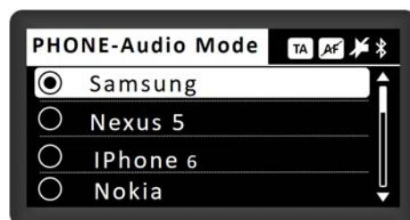
**PHONE-CONNECTED** main screen is shown when “Connected Devices” menu item is selected from the PHONE BROWSE screen. There are 2 different modes for connecting Bluetooth devices;
