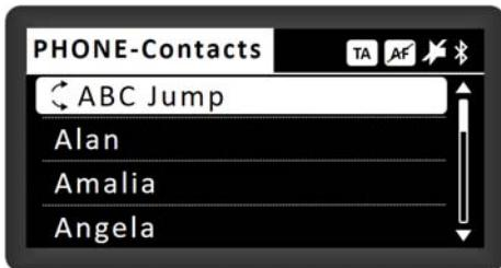
**PHONE-CONTACTS** can be seen by entering "Contacts" menu item. During new pairing process, or connection in-process (after radio turns on, it takes up to 20 seconds to connect already paired phones), "Loading, Please Wait" warning will be shown, until whole phonebook is downloaded to the radio.
