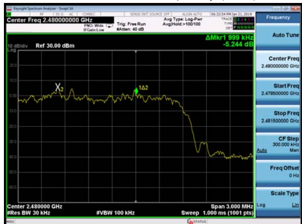
BT 2DH5 CH78, Carrier frequency (MHz): 2480
