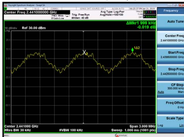
BT DH5 CH78, Carrier frequency (MHz): 2480
