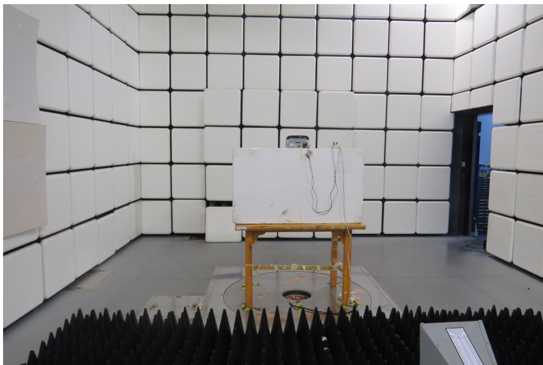
Picture 2 Radiated Emission Test Setup
