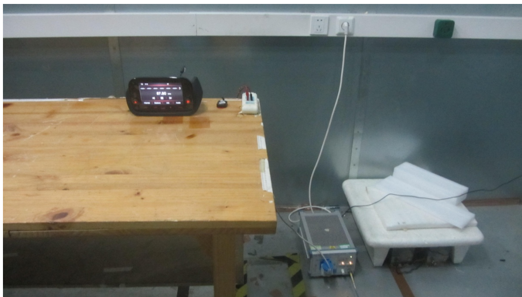
Picture 3 Conducted Emission Test Setup
