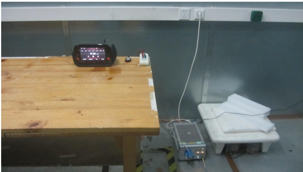
Picture 3 Conducted Emission Test Setup
