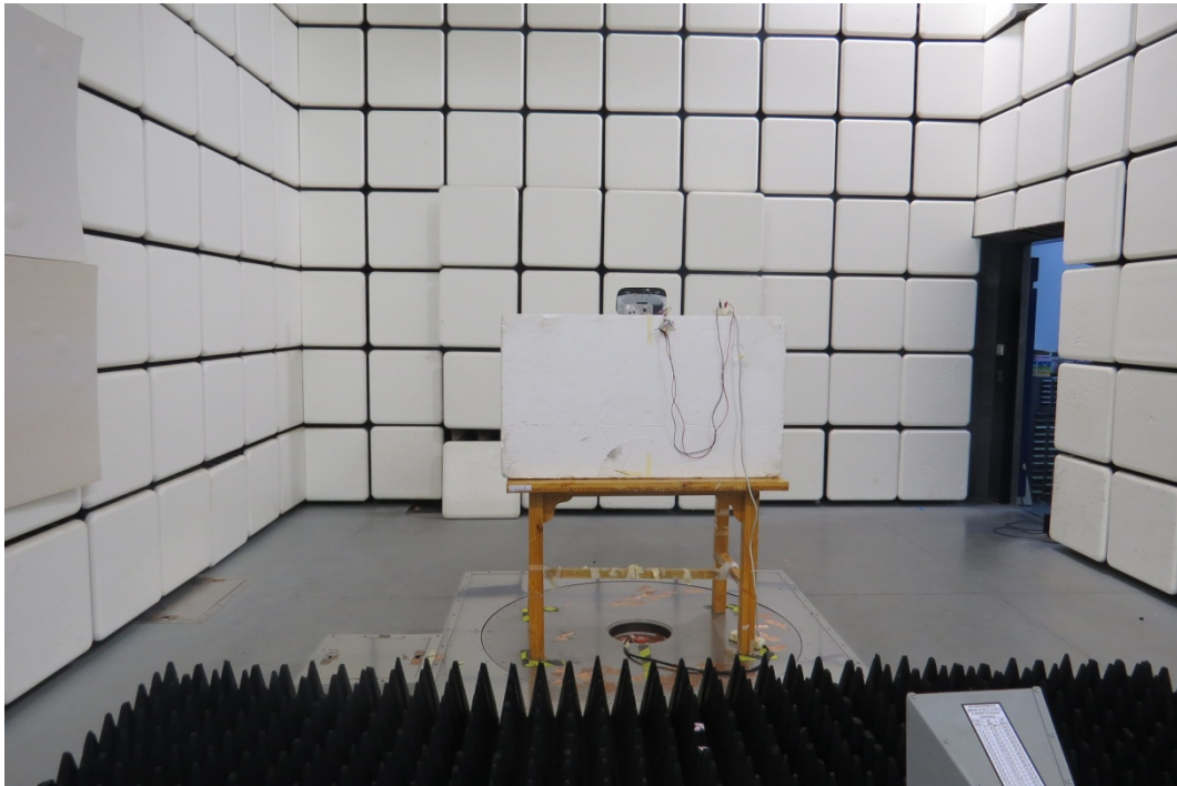
Picture 2 Radiated Emission Test Setup
