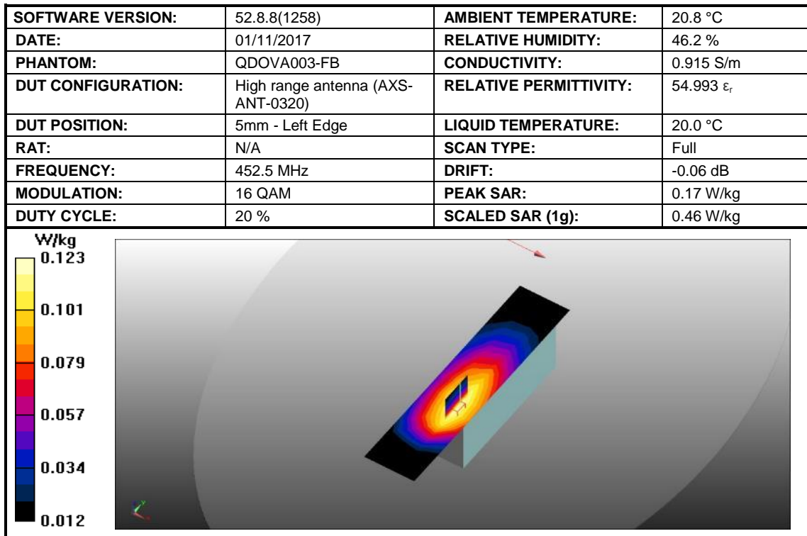
Figure 13: SAR Body Testing Results for PNG MP50 Transceiver at 452.5 MHz.
