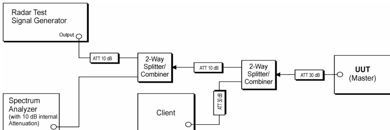
(Example Conducted Setup where UUT is a Master and Radar Test Waveforms are injected into the Master)
