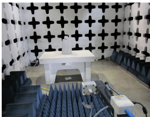
Radiated emissions test set up above 18GHz.
