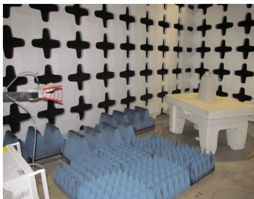
Radiated emissions test set up above 1GHz.
