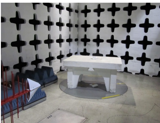
Radiated emissions test set up in 30MHz-1GHz frequency range
