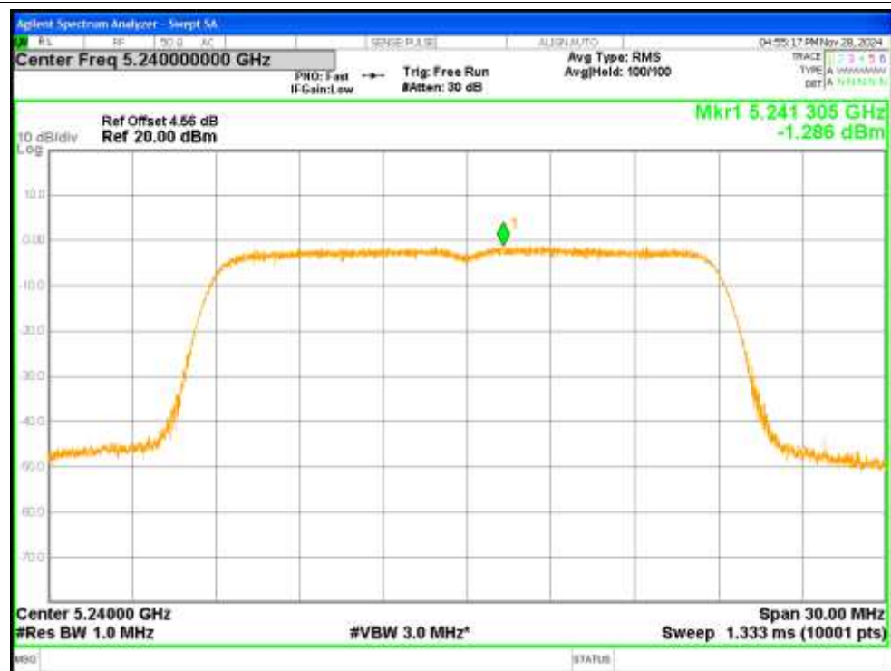
PSD NVNT n20 5240MHz Ant2
