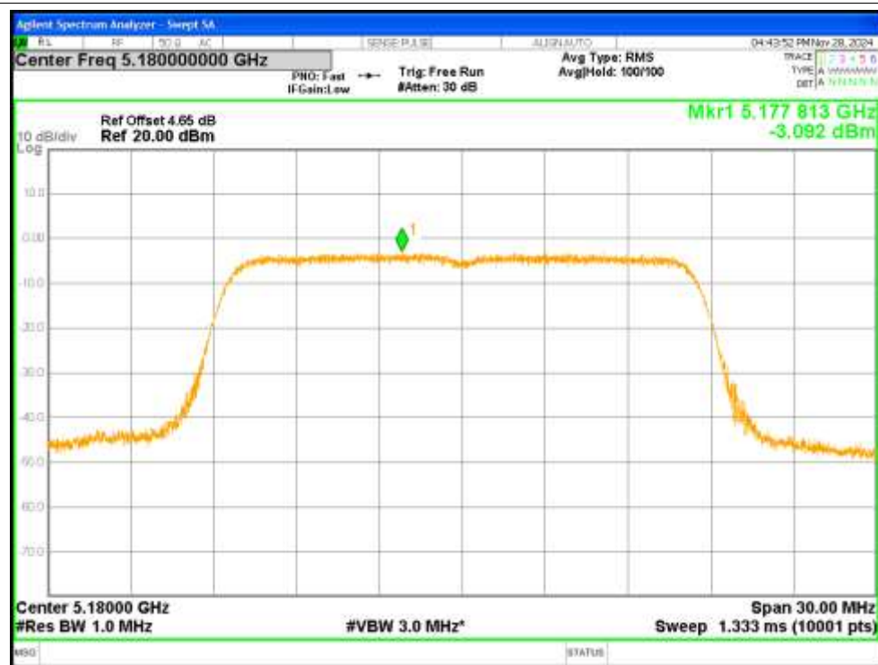
PSD NVNT a 5180MHz Ant2
