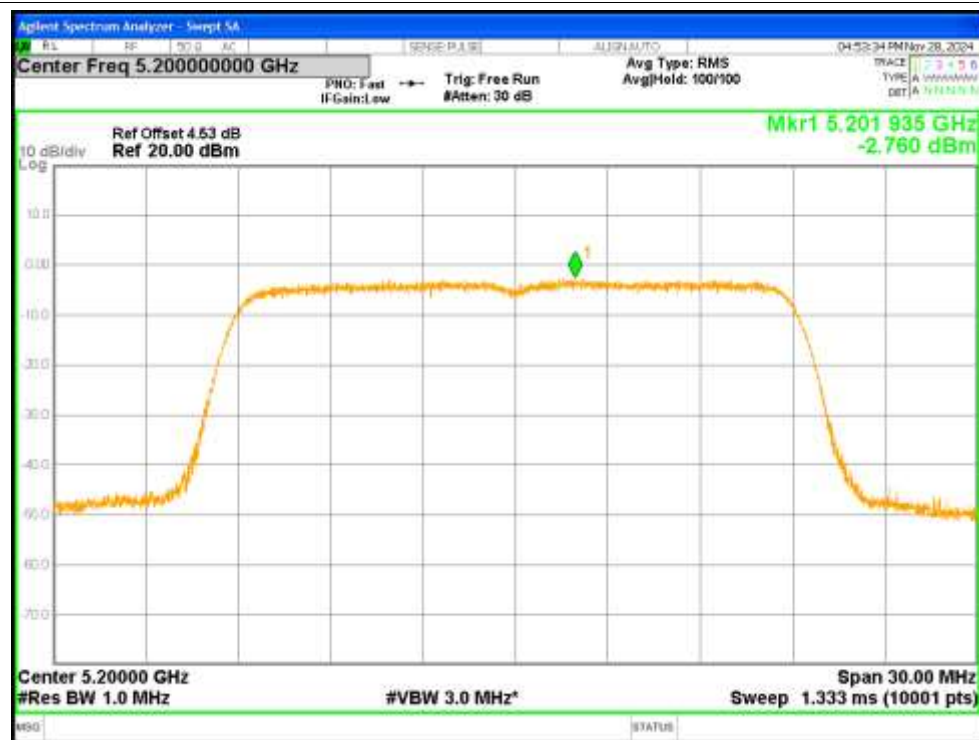
PSD NVNT n20 5200MHz Ant2
