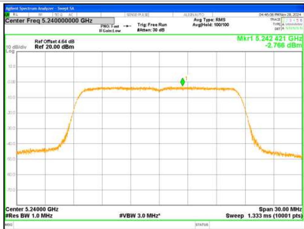
PSD NVNT a 5240MHz Ant2
