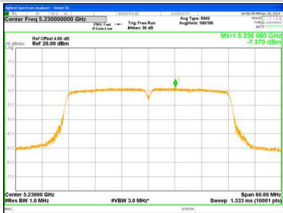
PSD NVNT n40 5230MHz Ant2
