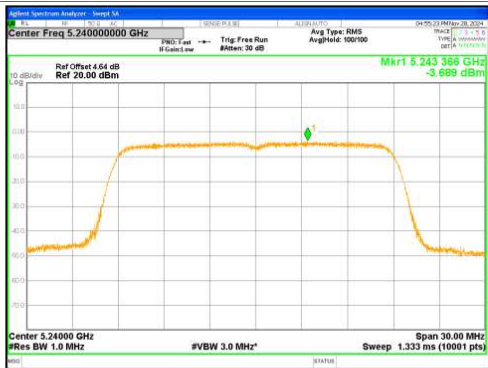
PSD NVNT n20 5240MHz Ant2
