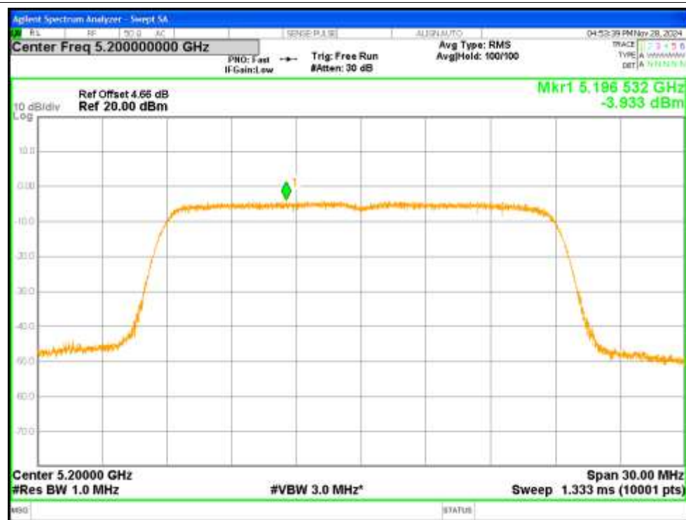
PSD NVNT n20 5200MHz Ant2
