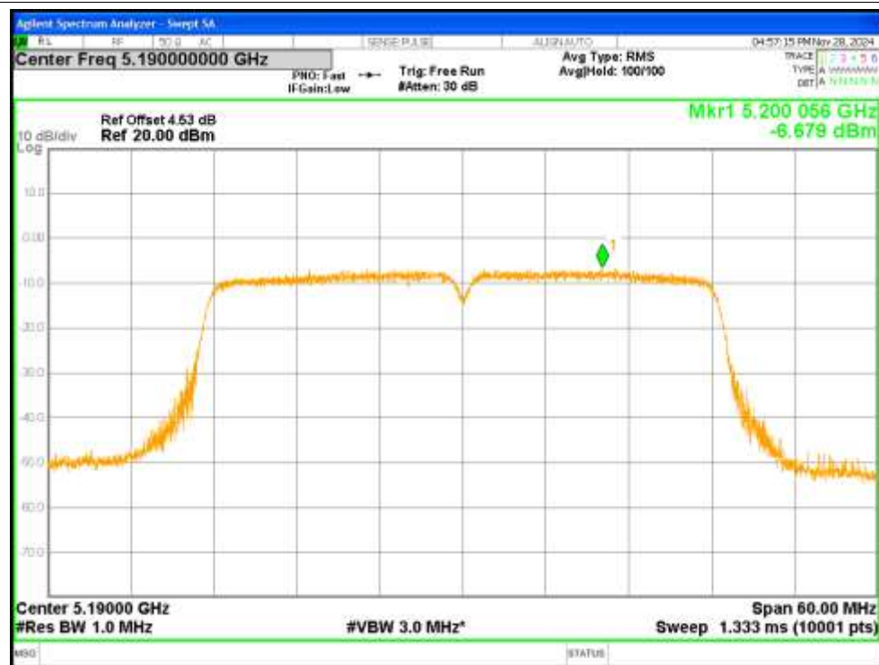
PSD NVNT n40 5190MHz Ant2
