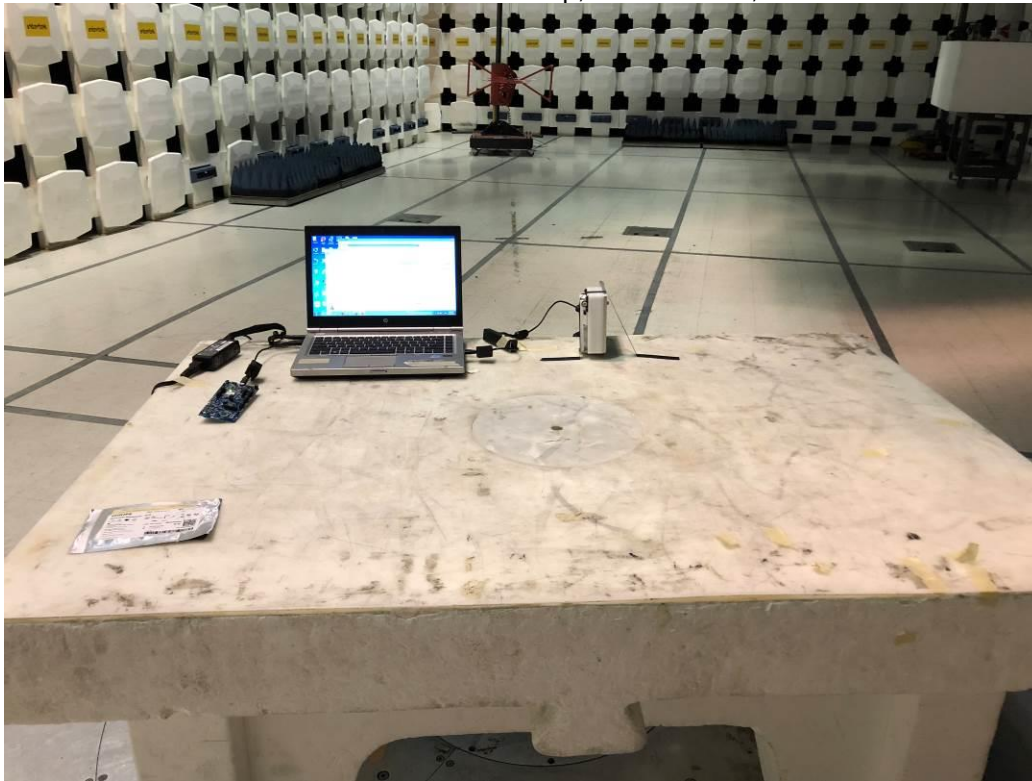
Radiated Emissions Test Setup, 30-1000 MHz, Y-axis
