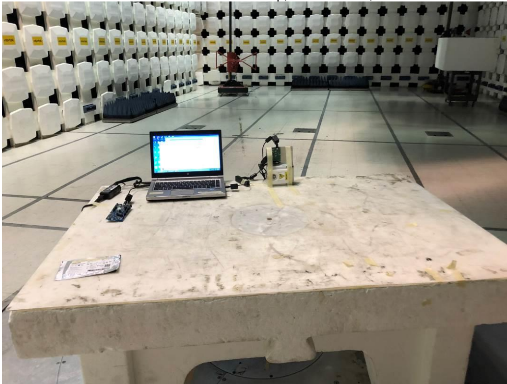
Radiated Emissions Test Setup, 30-1000 MHz, Z-axis
