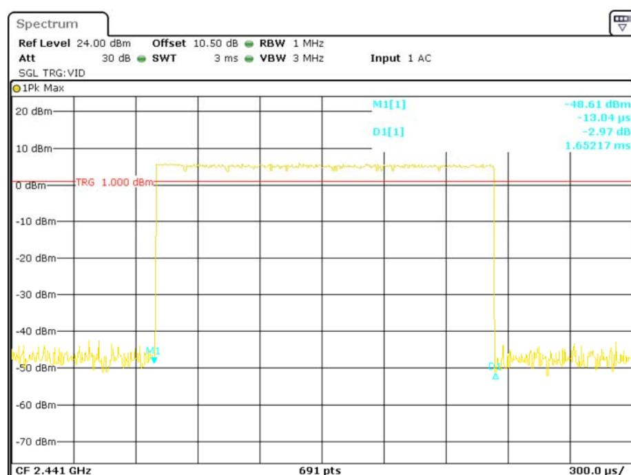
**Pulse time, High Channel, 2DH3**
