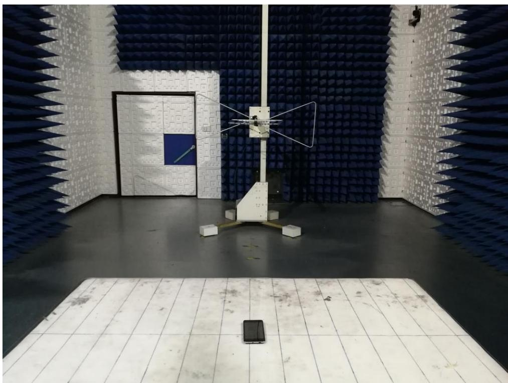
RADIATED EMISSION ABOVE 1G TEST SETUP
