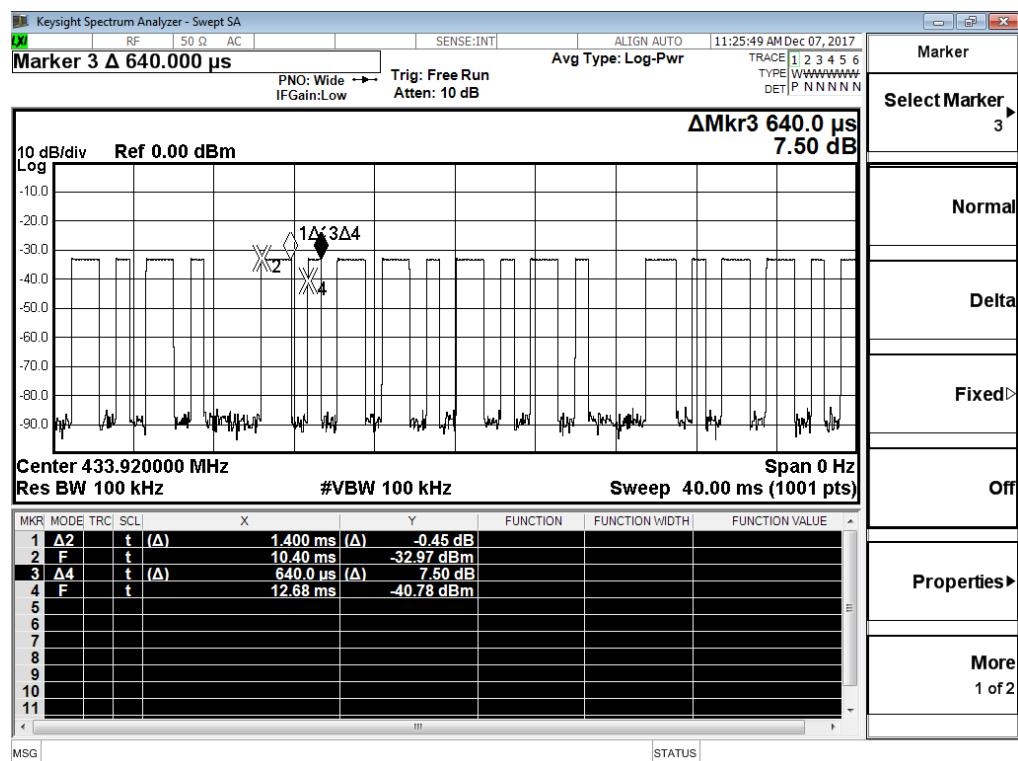
Pulse width (1.4ms) Pulse narrow(0.62ms)
