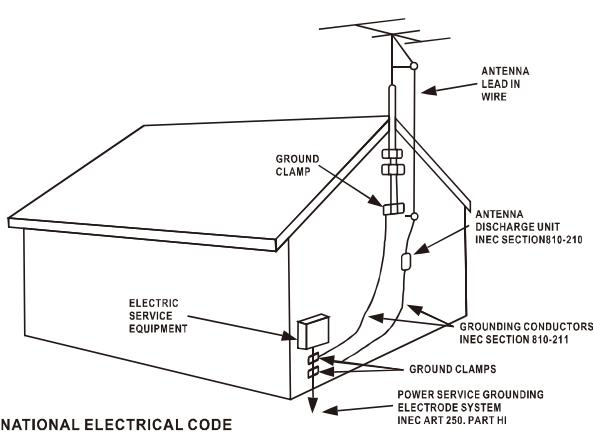
17. **POWER LINES** - An outside antenna system should not be located in the vicinity of overhead power lines or other electric light or power circuits, or where it can fall into such power lines or circuits. When installing an outside antenna system, extreme care should be taken to keep from touching such power lines or circuits as contact with them might be fatal.
