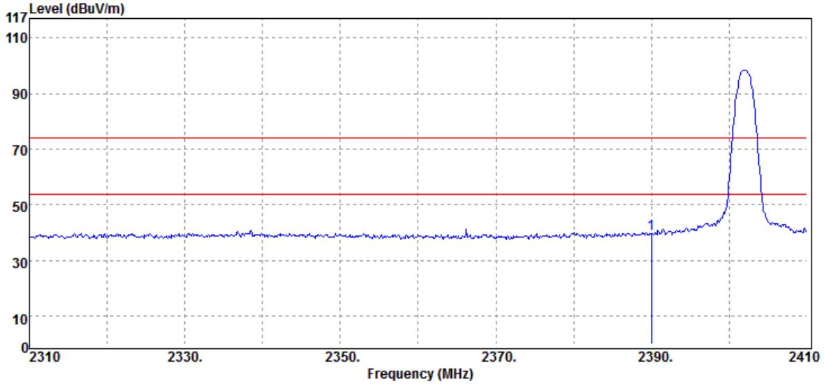
The plot shows the Level (dBuV/m) on the y-axis (0 to 117) versus Frequency (MHz) on the x-axis (2310 to 2410). A blue line represents the measured signal, which is relatively flat around 35 dBuV/m until approximately 2390 MHz, where it rises sharply to a peak of about 95 dBuV/m. Two horizontal red lines indicate the test limits: a lower one at approximately 52 dBuV/m and an upper one at approximately 74 dBuV/m.
