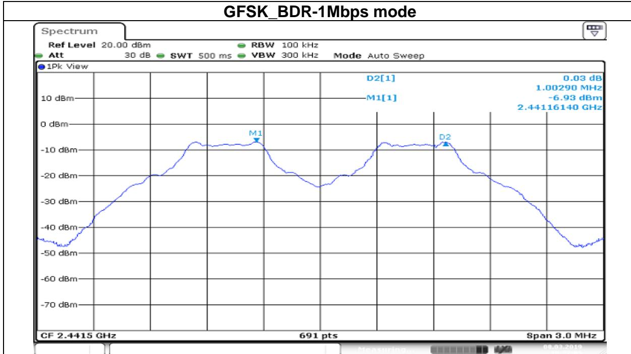
**Note:** We selected worst case to performed test in middle channel, The results can be meet other channel.
