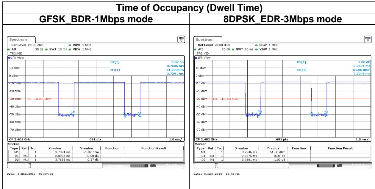
**Note:** We selected worst case to performed test in low channel. The results can be meet other channel.
