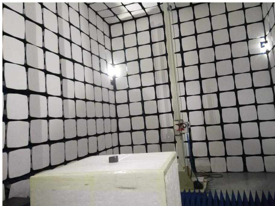
**Radiation Emission Test Setup (Above 18GHz)**
