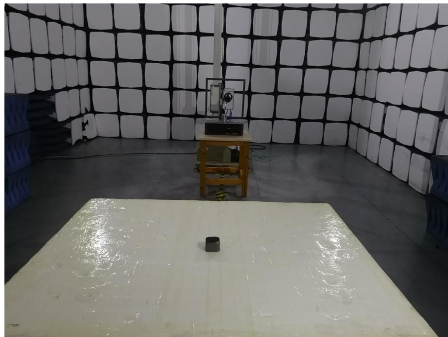
**Radiation Emission Test Setup (30MHz to 1GHz)**
