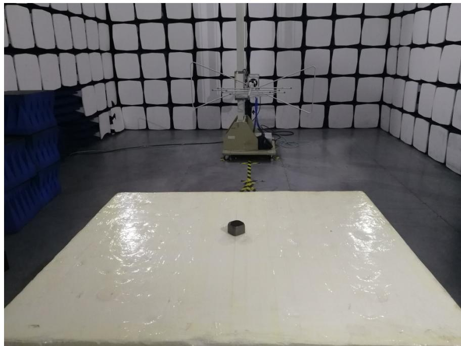
**Radiation Emission Test Setup (1GHz to 18GHz)**
