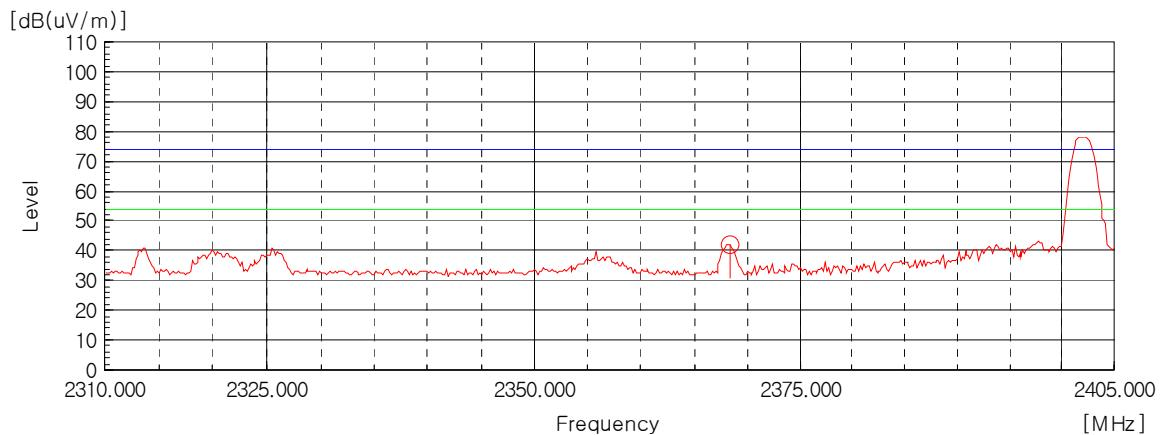
AV Detector: RBW: 1 MHz, VBW: 10 Hz (2 310 MHz - 2 390 MHz), Worst case (Low, Horizontal)
