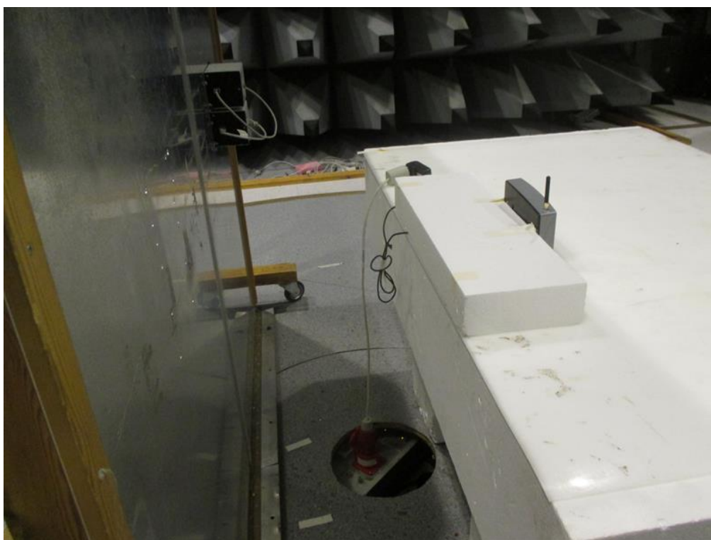
Photo 4.1.2 Test setup regarding measurement of radio frequency voltage on mains.
