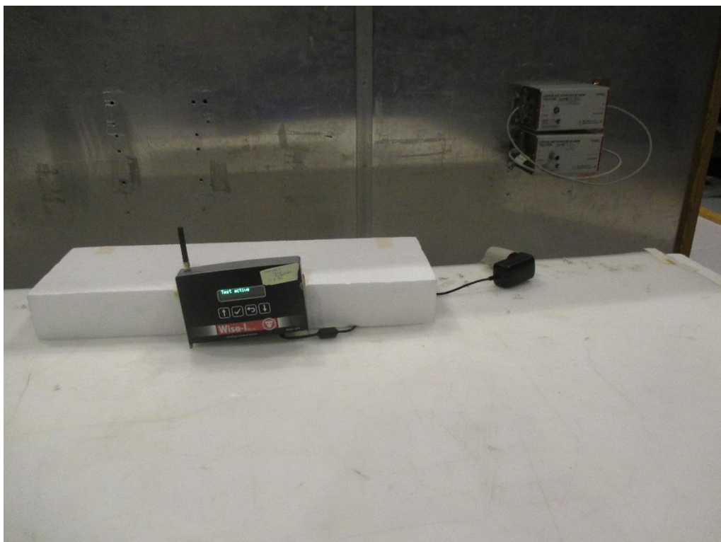
Photo 4.7.1 Test setup regarding measurement of radio frequency voltage on mains.
