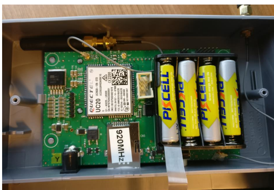
Figure 2: Shows the back side of the PCB mounted in the main enclosure
