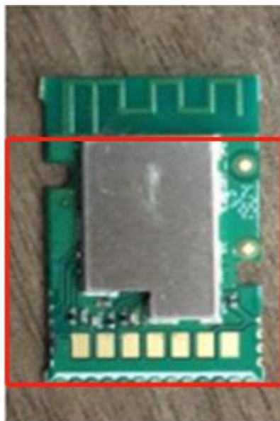
Drawing 2-3 Description of Clear Area of Antenna
