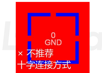
Figure 4.3 Copper connection not recommended
